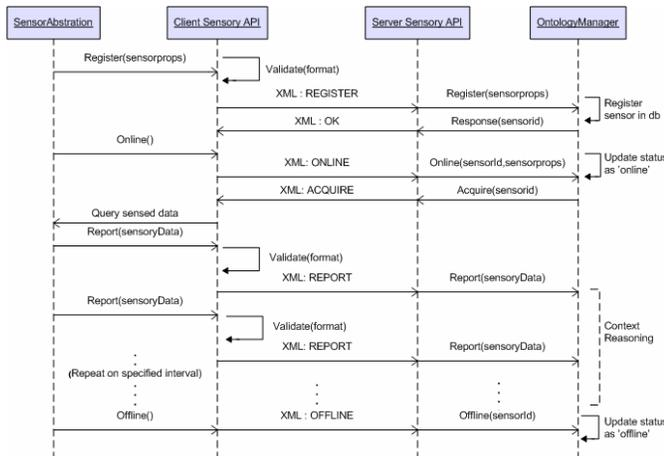
Figure 5. Typical sequence of operation of an ‘active’ sensor
