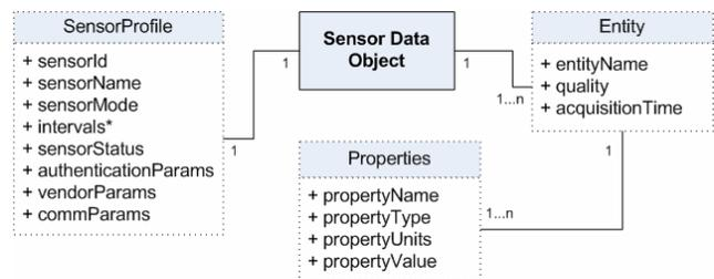
Figure 4. Sensor Data Model
