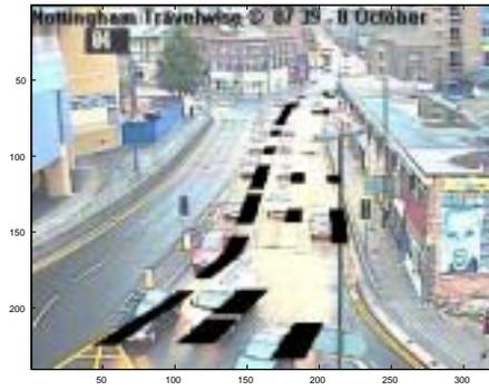
**Figure 13. Detected car regions for the head light case**
