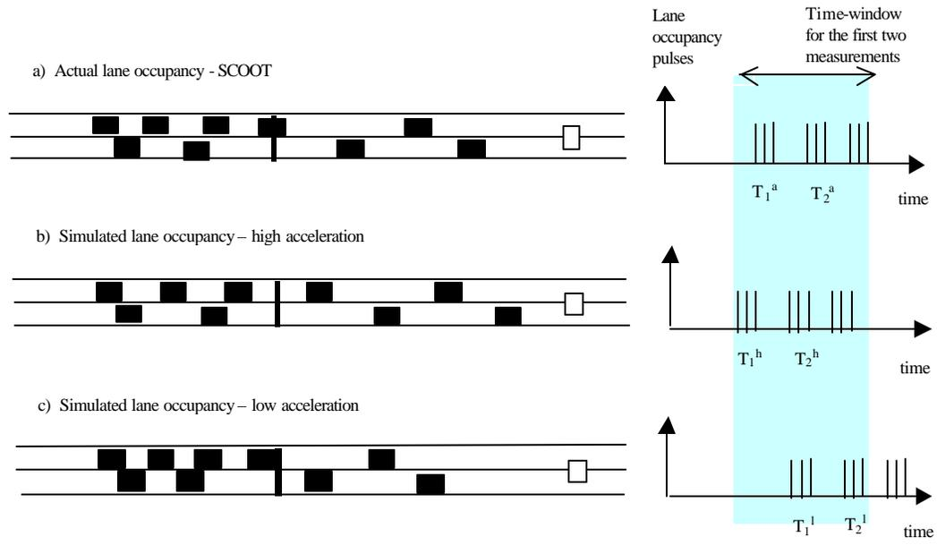
Figure 3. Actual and simulated lane occupancy with their corresponding measurements
