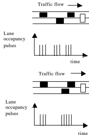
Figure 1. Real-time traffic measurements with 2-lanes inductive loops
