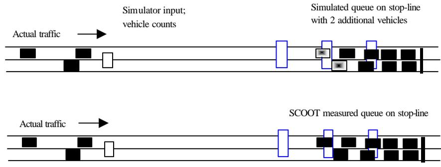
Figure 2. Correction of the systematic error in real-time simulations
