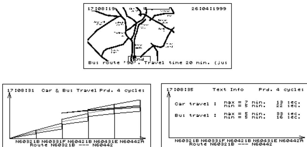
Figure 7. PSION-based interface to the mobile traffic/travel information client
