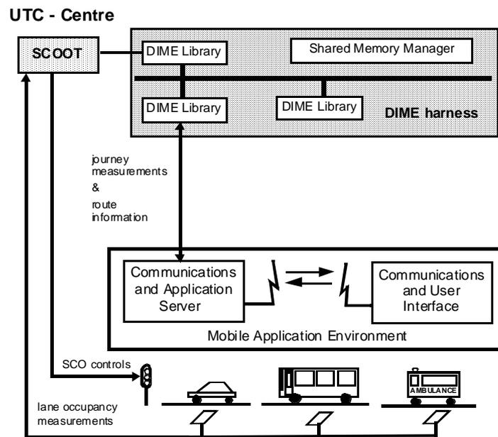
**Figure 4.** DIME interface to a portable traffic/travel information system
