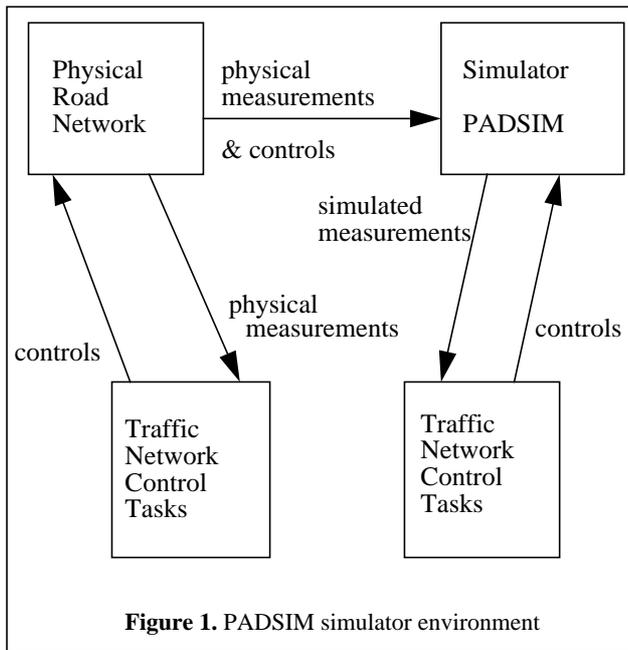
and the second one controls the simulated network. Such arrangement allows the PADSIM simulation to run ahead of real time. The traffic network control task acting on simulated measurements provides control sequences which effectively anticipate traffic situations thus assisting an operator in making appropriate supervisory controls.
