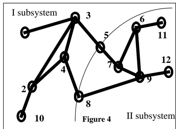
subnetworks are connected through “Boundary Nodes” (figure 4). For the example of Figure 4. the network is divided into two subsystems. The first subsystem consists of nodes 1, 2, 3, 4, 5, 8, 10 and the road sections between them, while subsystem 2 consists of nodes 5, 8, 6, 7, 9, 11, 12 and the road sections between them. Nodes 1, 10, 5 and 8 are Boundary Nodes for the first
