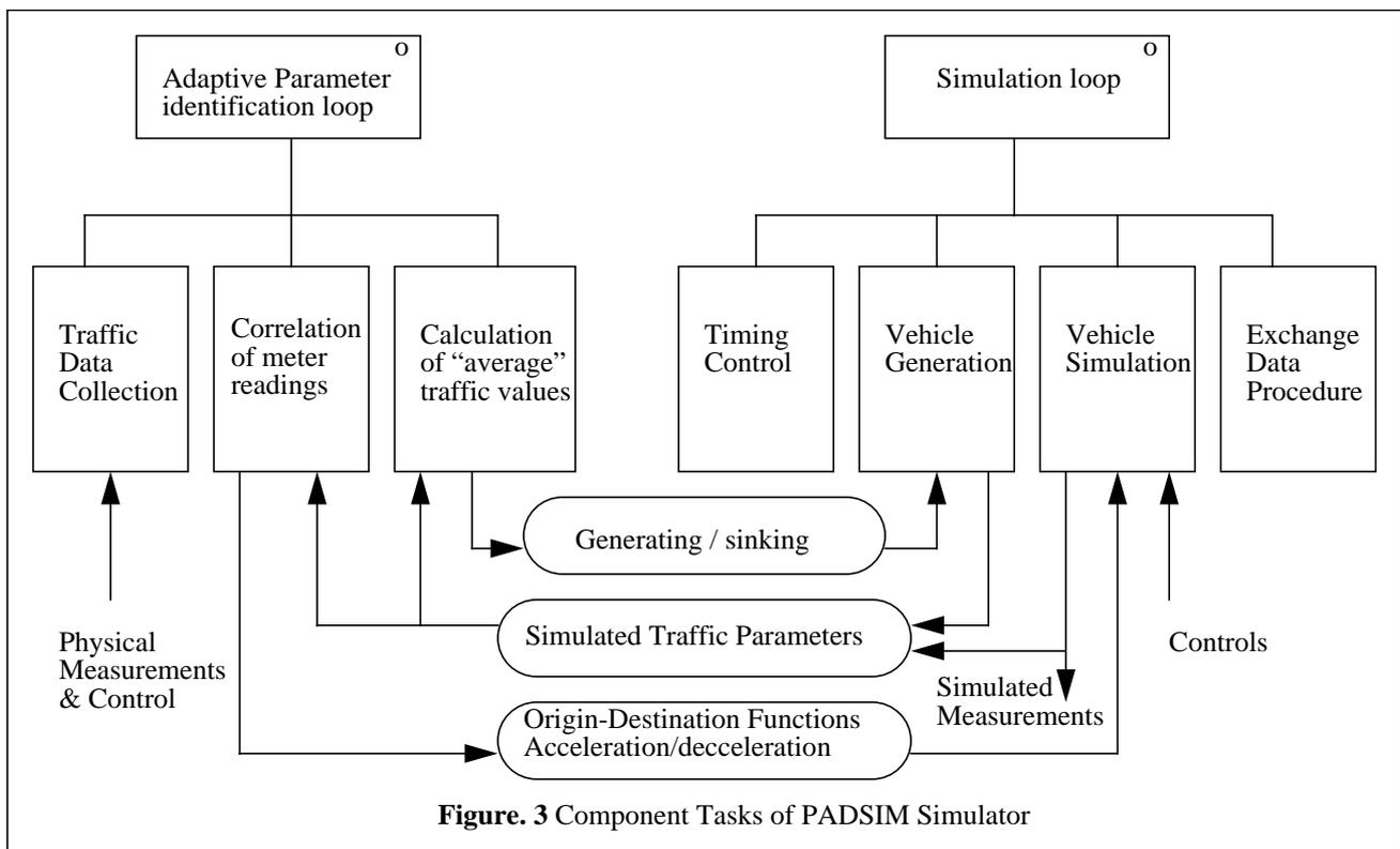
**Figure. 3** Component Tasks of PADSIM Simulator
