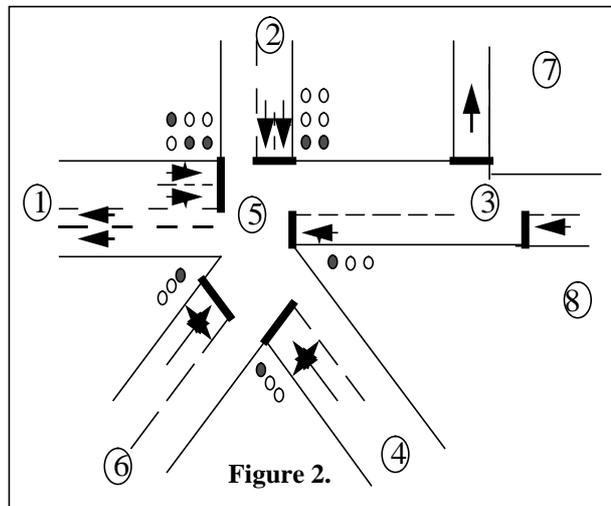
adjoining sections to these nodes is zero. Figure 2. illustrates a small network for which the nodes 1,2,4,6,7,8 are the Boundary Nodes, and nodes 3 and 5 are the Transit Nodes.
