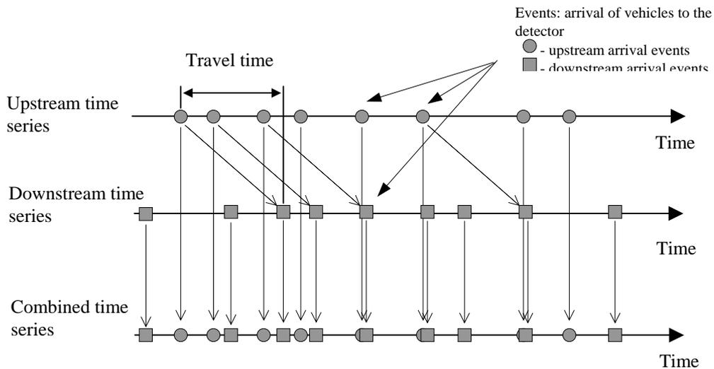
Figure 2. Merging upstream and shifted downstream time series
